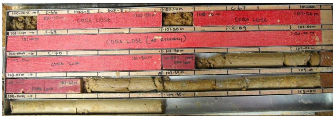
**Figure 4:** Drill cores obtained from borehole HTS-5 (see Figure 3) from the tunnel level with a triple-tube core barrel. The borehole penetrated the tunnel at around Ch. 750 (compare Fig. 5 and Table 1 for actual geology at Ch. 750).
