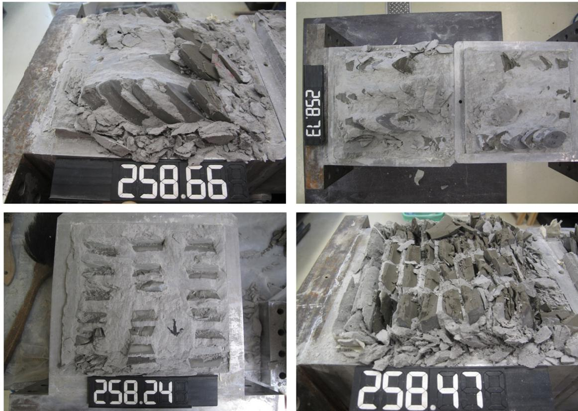
**Figure 2: Failure surfaces after the test shown for 30° block proportion (top left and right), 90° block proportion (bottom left) and 60° block proportion (bottom right).**
