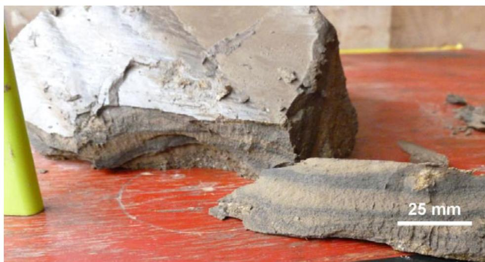
**Figure 8: Brownish-blackish matrix material with slickensides (left) and layering (right). The slickensides were presumably generated by deformations ahead of the face (Ch. 735) and not by tectonic processes. The layering may indicate previous internal tectonic deformation of shear lenses in the fault core.**
