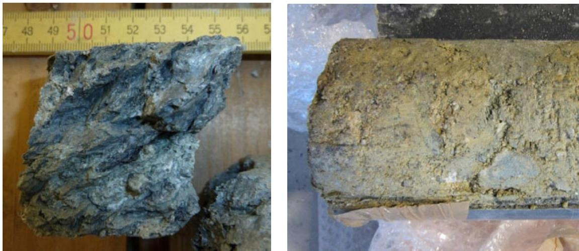
**Figure 1: Examples of typical testing material; cataclasites from phyllite and schist. The material can easily be broken by hand.**
