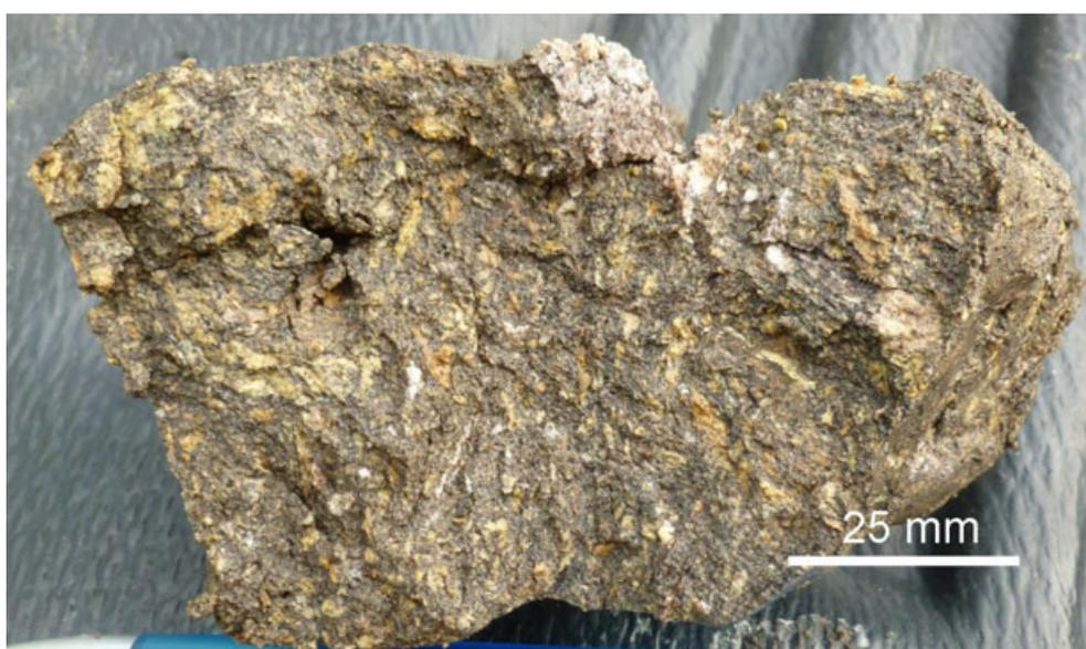
**Figure 7: Lump of brownish-blackish undisturbed matrix soil of the fault core (Ch. 730). The material feels similar to damp compacted peat. For grain size distribution and NMC see Table 2.**
