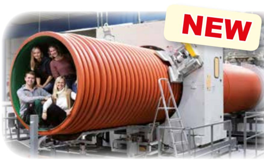
We produce the PP-MEGA-pipe DN/ID 1600 with an outside diameter of approx. 1800 mm.
